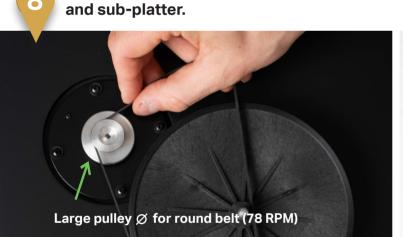
Put the flat drive belt (c) on the pulley
