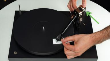
When the gauge stays level, your tracking force is set correctly. \*identical with Sumiko Rainier
